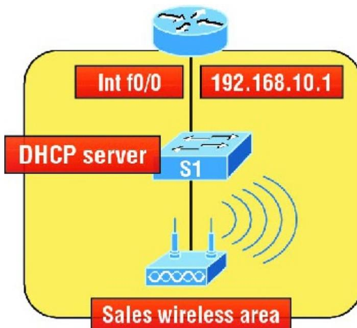
**FIGURE 7.2** DHCP configuration example on a switch
