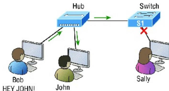
**FIGURE 1.2** A switch can break up collision domains.
