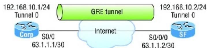
**FIGURE 21.24** Example of GRE configuration
