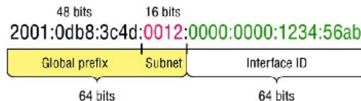
**FIGURE 14.1** IPv6 address example
