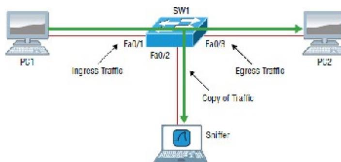
**Figure 20.2** Using SPAN for troubleshooting
