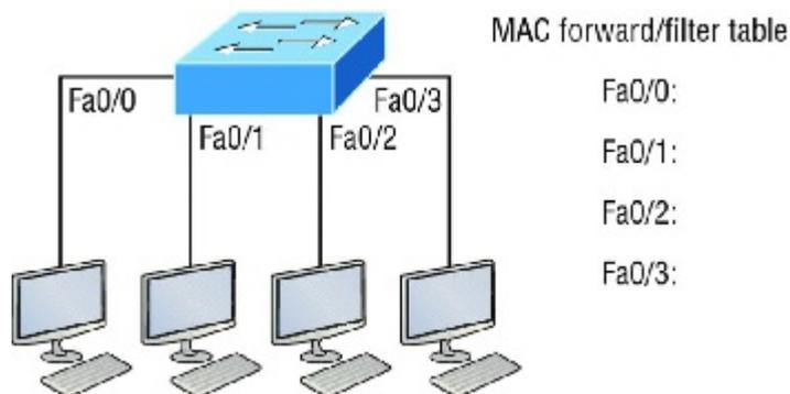
**FIGURE 10.1** Empty forward/filter table on a switch
