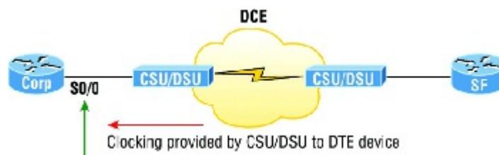
**FIGURE 21.11** Configuring Cisco's HDLC proprietary WAN encapsulation
