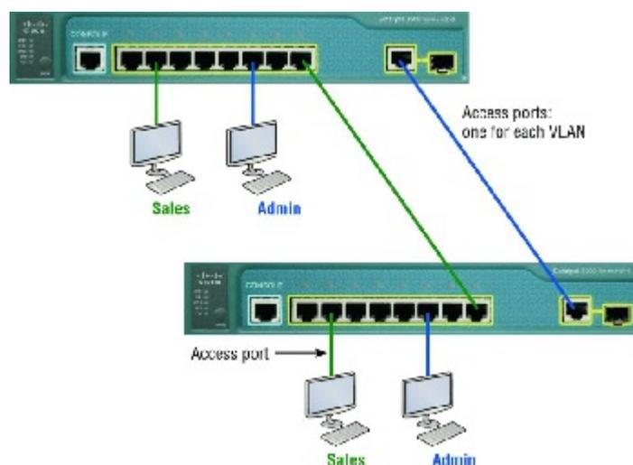
**FIGURE 11.5** Access ports
