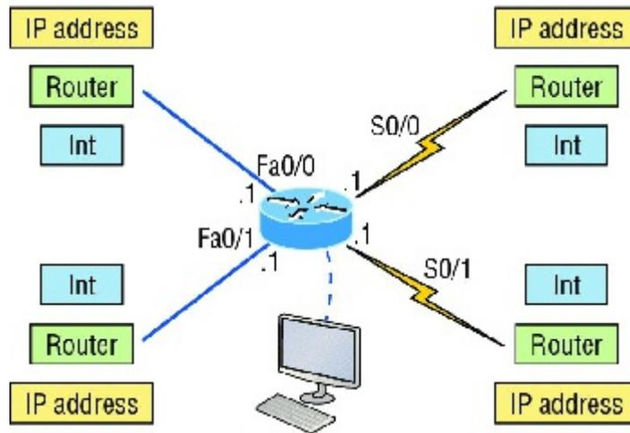
**FIGURE 7.7** Documenting a network topology using CDP
