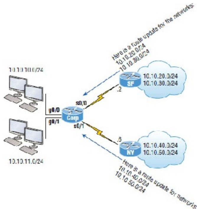
**FIGURE 17.8** Split horizon in action, part 1
