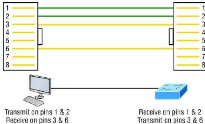
**FIGURE 2.10** Straight-through Ethernet cable
