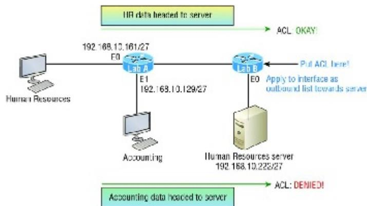
**FIGURE 12.3** IP standard access list example 2
