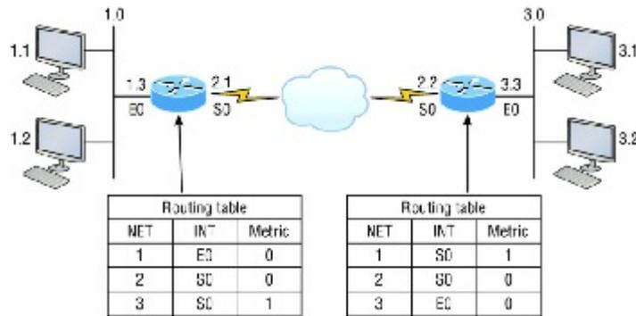
**FIGURE 1.14** Routing table used in a router
