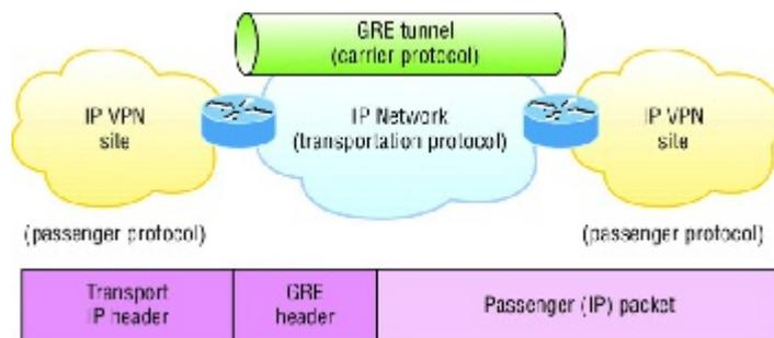
**FIGURE 21.23** Generic Routing Encapsulation (GRE) tunnel structure
