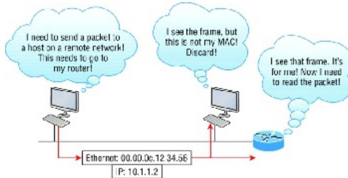
**FIGURE 3.23** Unicast address
