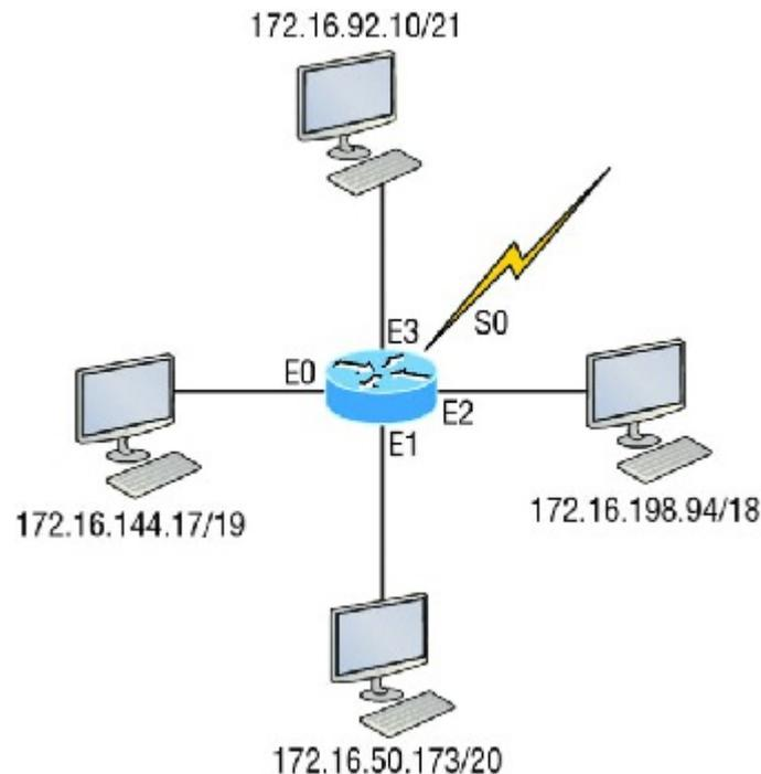
**FIGURE 12.4** IP standard access list example 3
