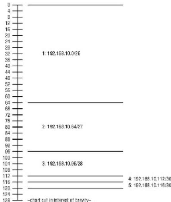
**FIGURE 5.11** Solution to VLSM design example 2
