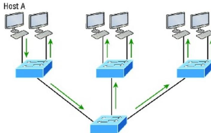
**FIGURE 11.1** Flat network structure
