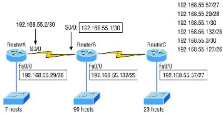
**FIGURE 5.9** Solution to VLSM design example 1
