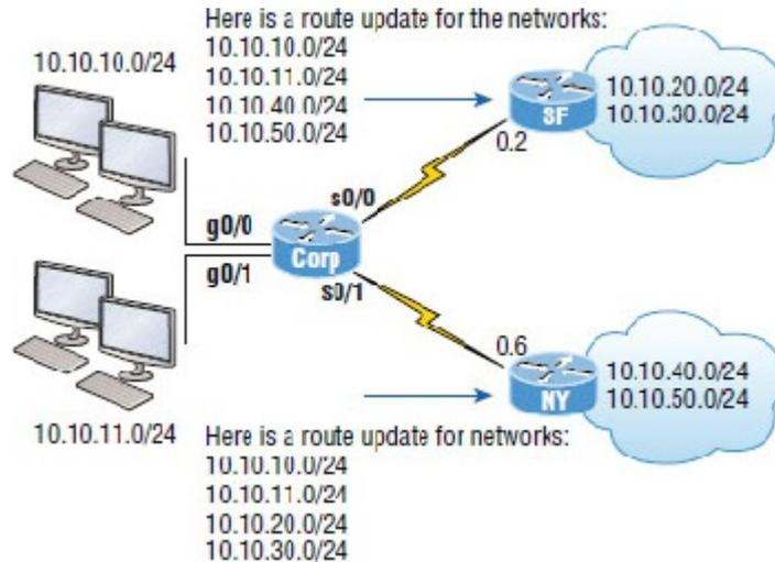
**FIGURE 17.9** Split horizon in action, part 2
