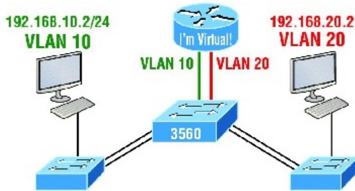
**FIGURE 11.16** Inter-VLAN routing with a multilayer switch
