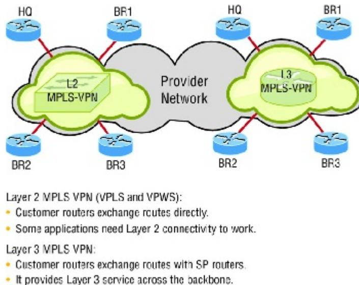
**FIGURE 21.22** Provider-managed VPNs
