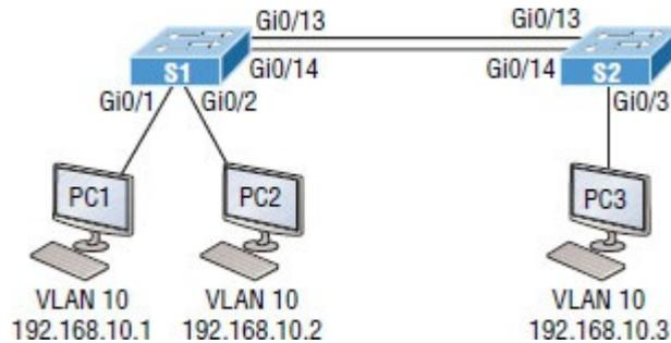
**Figure 20.7** VLAN connectivity
