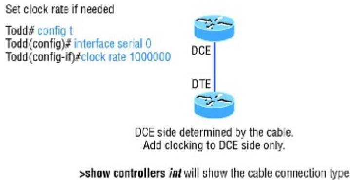
**FIGURE 6.4** Providing clocking on a nonproduction network
