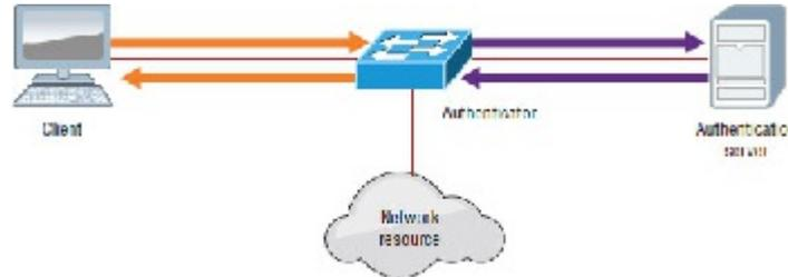
**Figure 16.3** Identity-based networking
