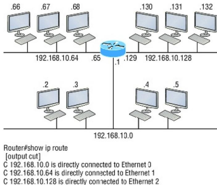
**FIGURE 4.4** Implementing a class C /26 (with three networks)
