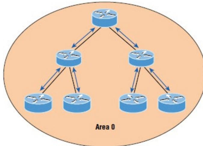
**Figure 19.1** OSPF single-area network: All routers flood the network with link-state information to all other routers within the same area.
