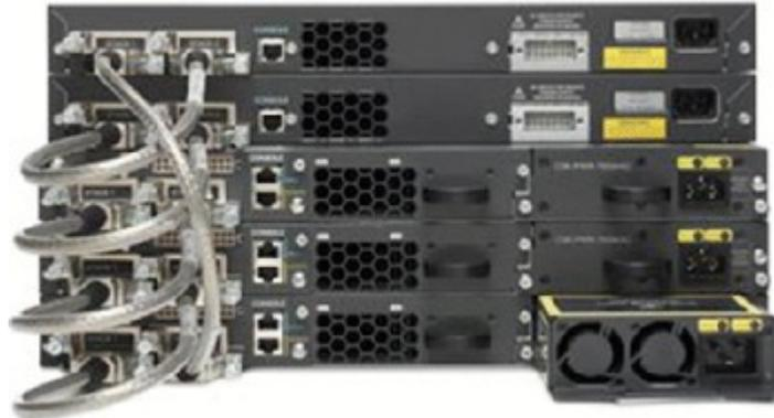
**FIGURE 22.1** Switch stacking
