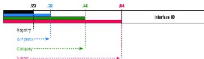
**FIGURE 14.2** IPv6 global unicast addresses
