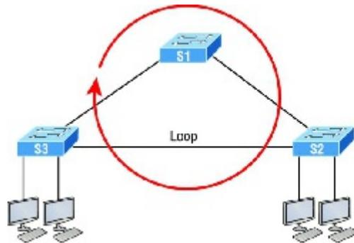
**FIGURE 15.2** A switched network with switching loops
