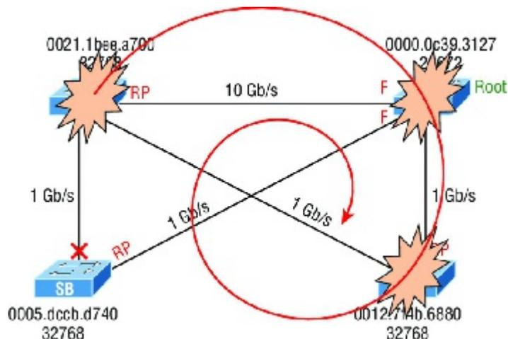
**FIGURE 15.18** STP failure
