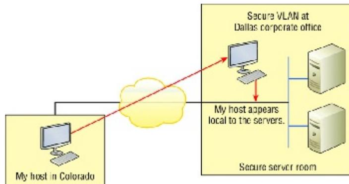
**FIGURE 21.20** Example of using a VPN
