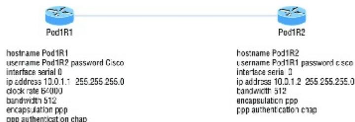
**FIGURE 21.15** Failed PPP authentication
