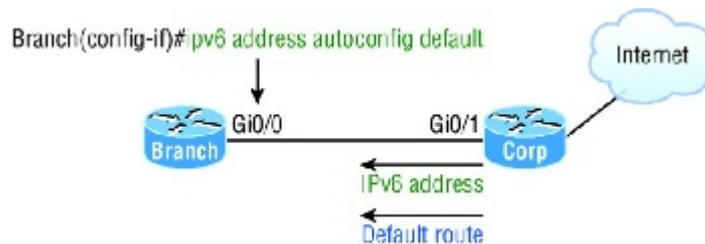
**FIGURE 14.6** IPv6 autoconfiguration example
