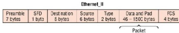
**FIGURE 2.8** Typical Ethernet frame format
