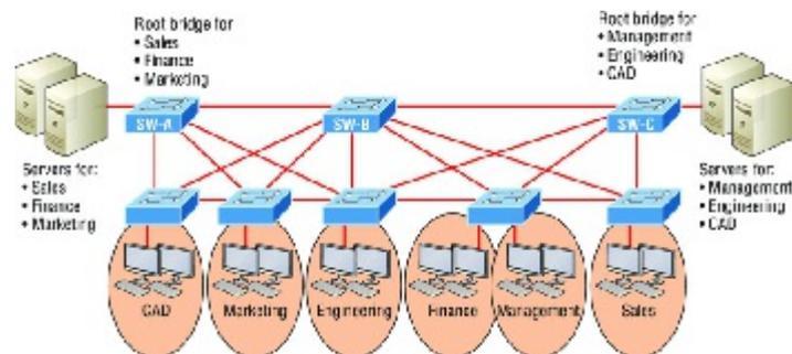
**FIGURE 15.9** PVST+ provides efficient root bridge selection.
