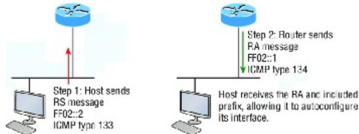
**FIGURE 14.5** Two steps to IPv6 autoconfiguration
