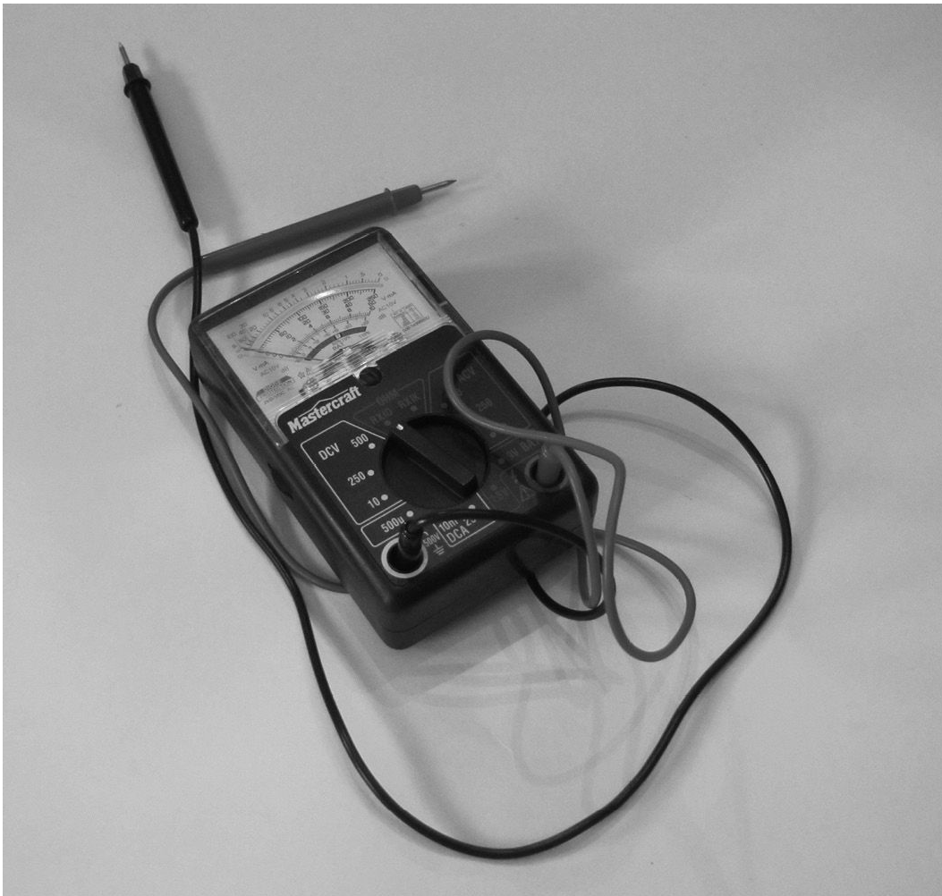
FIGURE 17-4 A multimeter can detect cable issues by measuring resistance.
