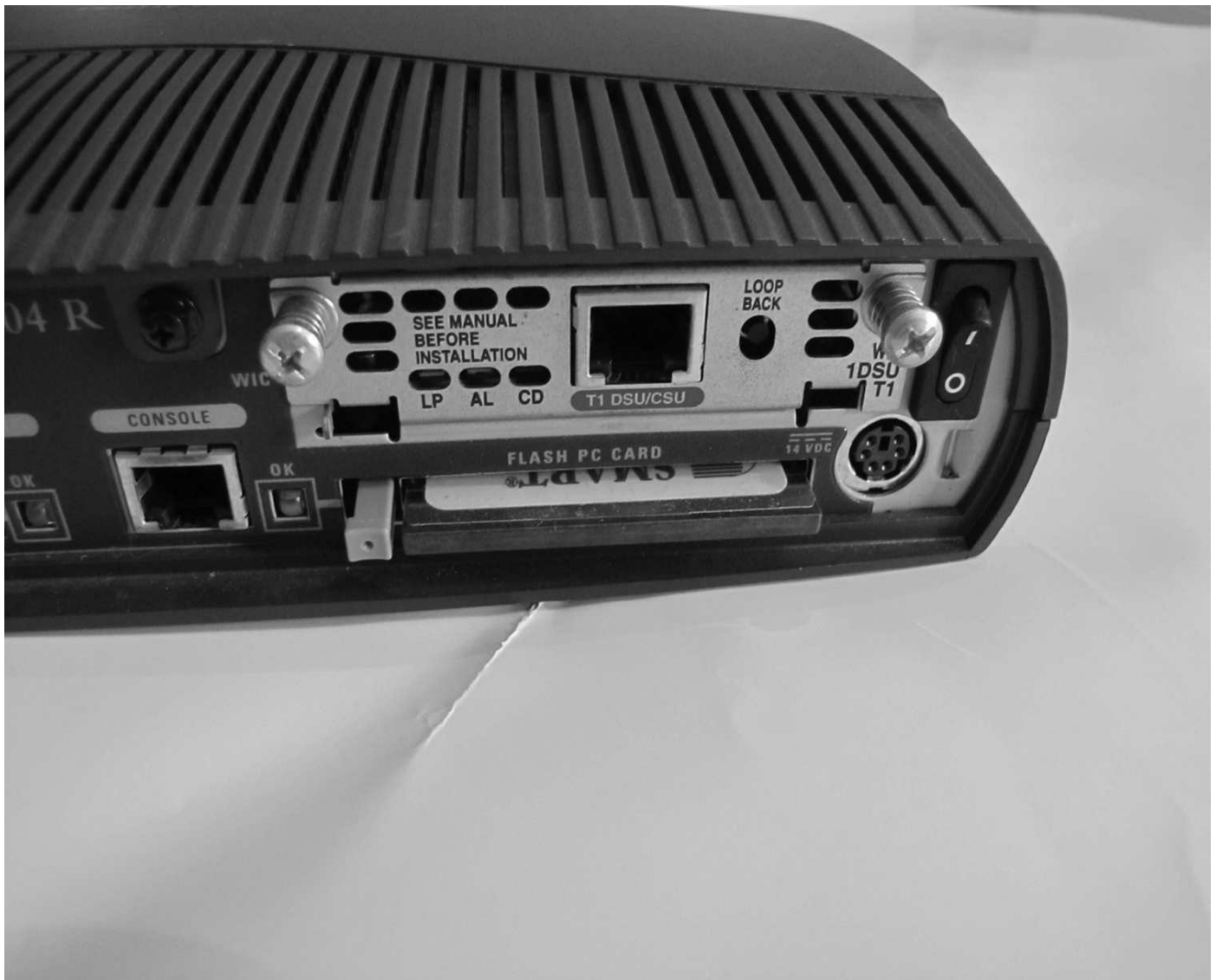
FIGURE 12-7 An integrated CSU/DSU on a router
