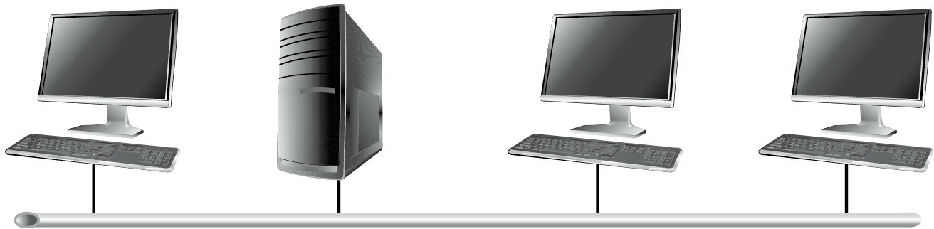
FIGURE 1-3 With a bus topology, all systems are connected to one linear cable.
