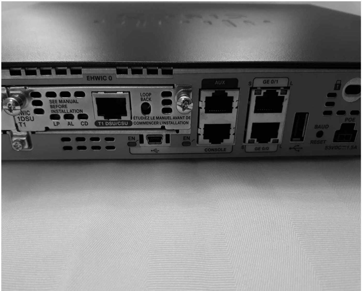
FIGURE 11-1 Console port and AUX port for out-of-band management
