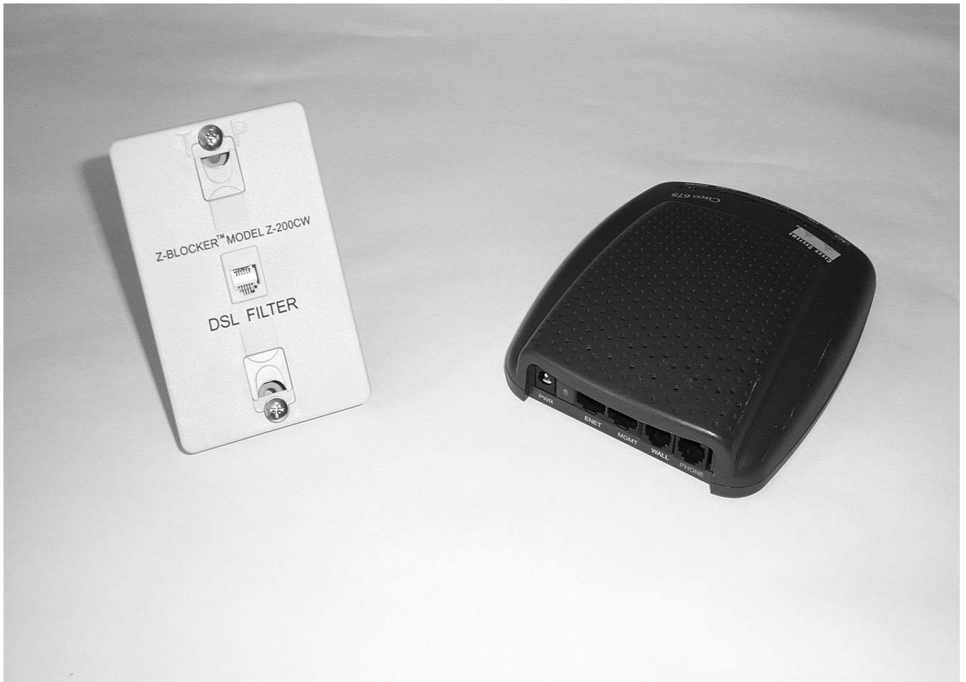
FIGURE 12-9 An ADSL frequency filter and an ADSL modem
