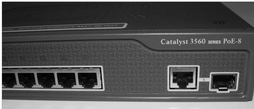
FIGURE 11.18 Switched Ethernet ports can provide power to devices.
