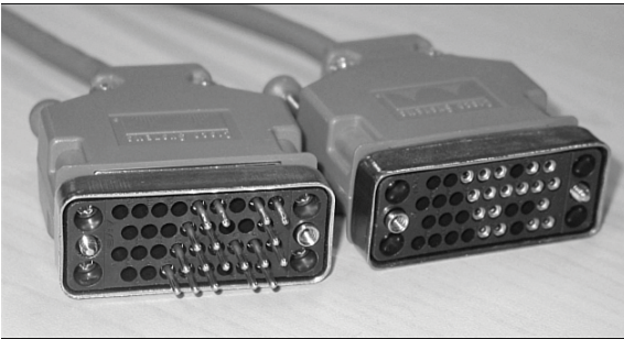
Figure 4-6 V.35 DTE and DCE Cables
